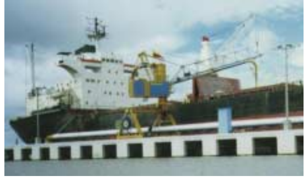
1990 : Colombia - Cartagena - 1 NIV 300 shipunloader on rails for unloading of bulk barley and malt with minimal breakage capacity : 300 MT/Hour
