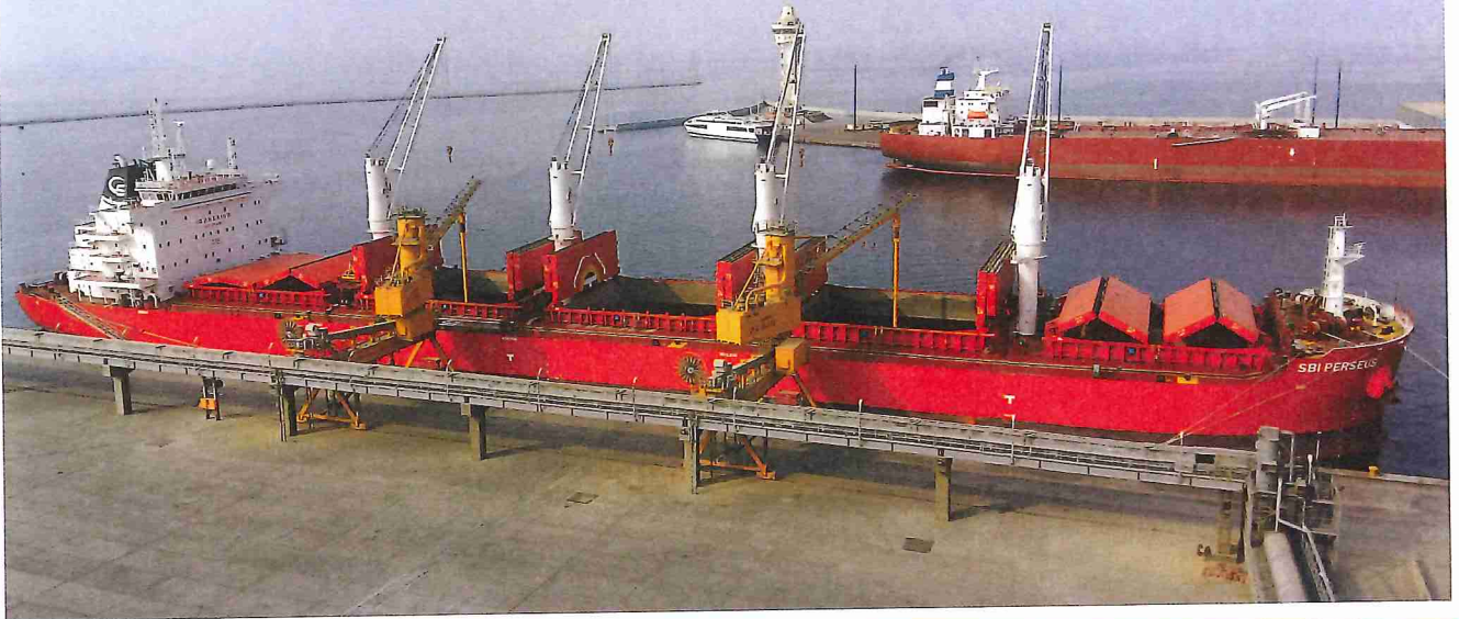
Two 600tph NIVs installed in Jazan.
