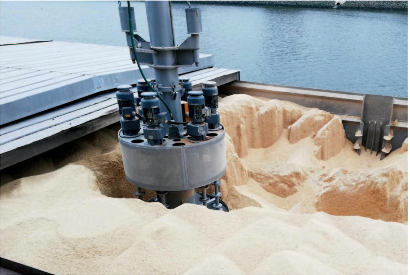
but also ‘new’ raw materials such as (D)DGS and rapeseed meal. With Vigan’s tailor-made cutting nozzles many agglomerating raw materials are gently dispersed for onward smooth pneumatic transport.
