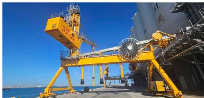
Figure 6. VIGAN CSU NIV 300 tph in Misurata, Libya.
