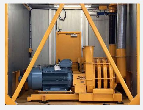
Another consequence of the use of inverters are to be noticed at the acoustic level. Thanks to the use of power adaptation in operation and multi-stage design, noise emissions are greatly reduced compared with other technologies such as root pumps. Additionally, VIGAN has developed custom noise cancelling solutions to reach low-noise emission values, which is especially useful in urban environments.
