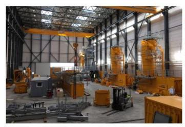
VIGAN has a 12,000-square-meter production facility that allows for premounting and full electrification, reducing assembly on site and the chance for errors.
